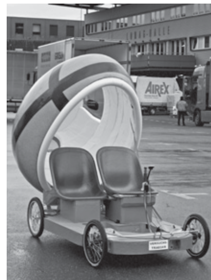
Fig. 2 Rolling platform with two seats under the open cabin
