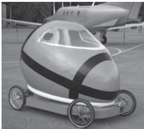
Fig. 1 UCV prototype with sandwich platform and helmet cabin
