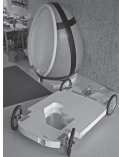
Fig. 3 Sandwich platform with EPS foam core and foam cabin
