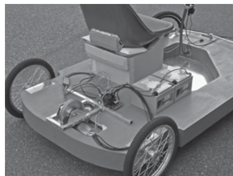
Fig. 4 Electric power train and batteries
