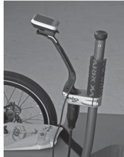
Fig. 7 Mechanical “joystick” with brake lever carrying display and sleeve for power control
