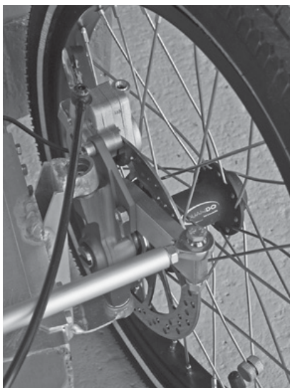
Fig. 6 Front wheel with disc brake and steering mechanics
