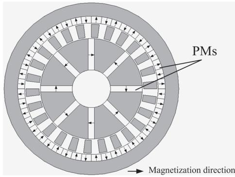
**Fig. 5** Magnetic gear with inner tangentially magnetized PMs
