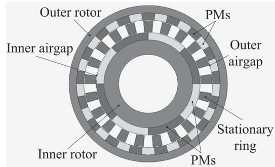
**Fig. 7** 2-D structure of magnetic gear
