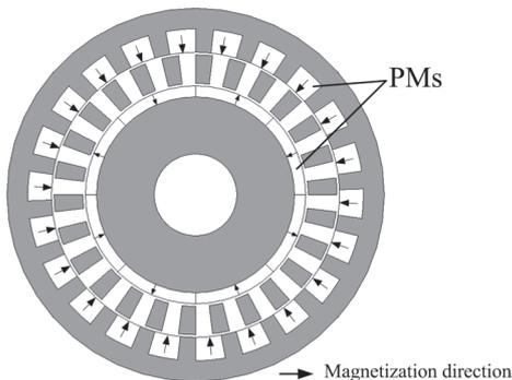
**Fig. 6** Magnetic gear with same polarity outer PMs
