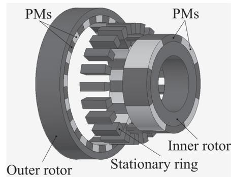
**Fig. 8** 3-D structure of magnetic gear
