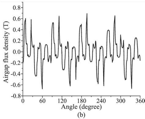
**Fig. 9** Airgap flux density waveforms of magnetic gear installed with Alnico: (a) inner rotor; (b) outer rotor
