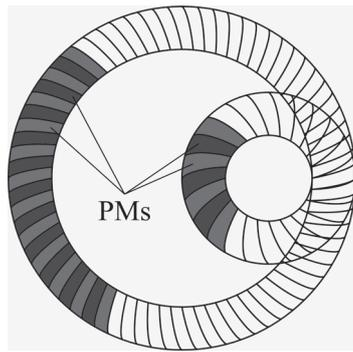
**Fig. 1** Involute SmCo magnetic gear
