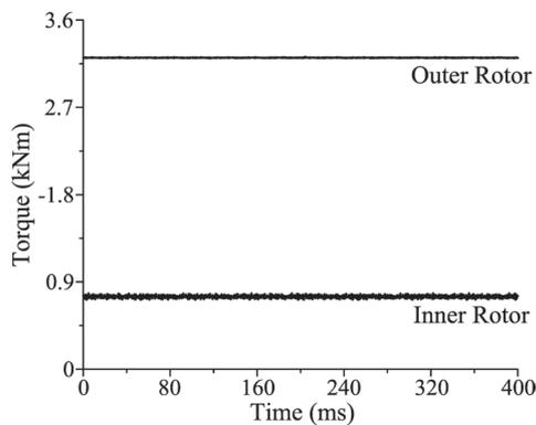
**Fig. 14** Torque waveforms of magnetic gear installed with SmCo
