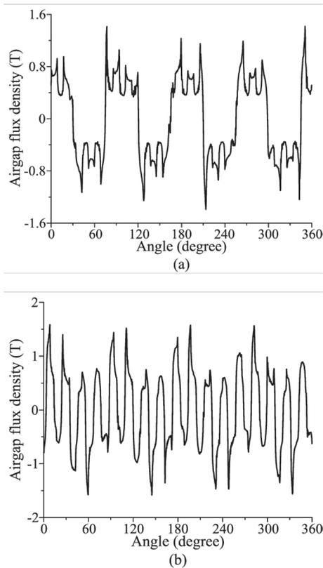
**Fig. 13** Airgap flux density waveforms of magnetic gear installed with SmCo: (a) inner rotor (b) outer rotor
