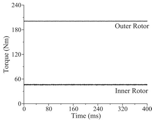
**Fig. 10** Torque waveforms of magnetic gear installed with Alnico
