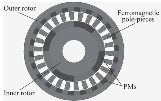
**Fig. 3** Coaxial magnetic gear
