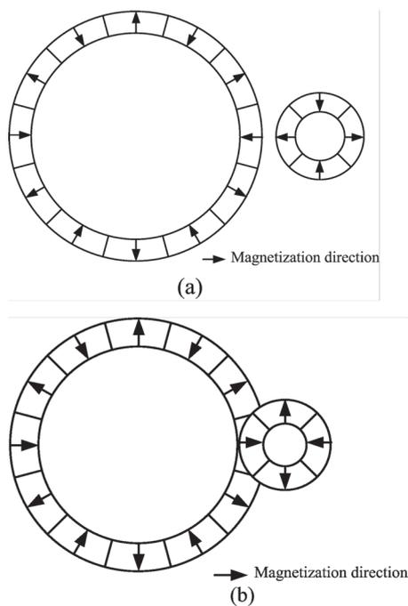
**Fig. 2** Parallel-axis magnetic gear: (a) radial-coupling; (b) axial-coupling
