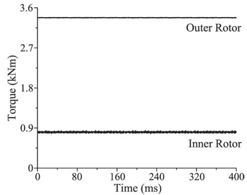
**Fig. 12** Torque waveforms of magnetic gear installed with NdFeB
