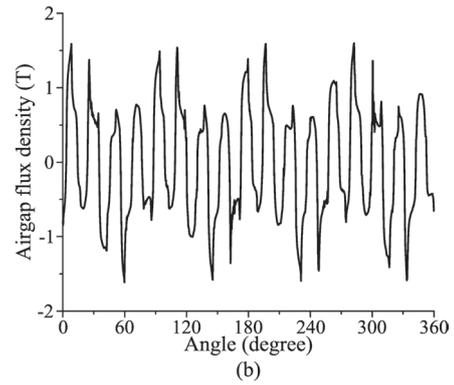
**Fig. 11** Airgap flux density waveforms of magnetic gear installed with NdFeB: (a) inner rotor; (b) outer rotor
