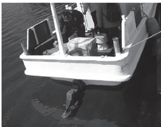
Fig. 4 A photograph of the stern electric drive of PHEB-2
