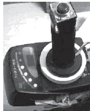
Fig. 9 The newly designed grip and base-area mounted on the joystick
