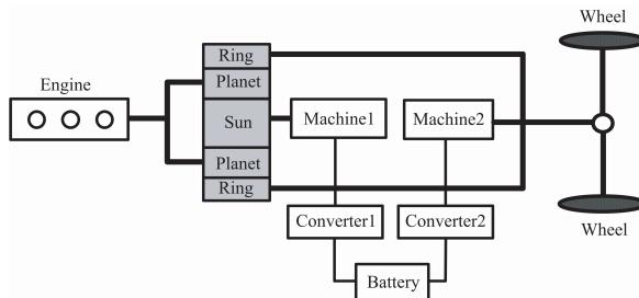
**Fig. 1** Toyota gear E-CVT propulsion system
