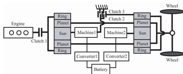
**Fig. 3** GM-Allison gear E-CVT propulsion system
