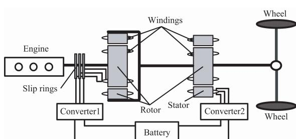
**Fig. 4** Double-rotor cascaded induction machine gearless E-CVT propulsion system
