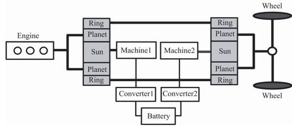
**Fig. 2** Ford gear E-CVT propulsion system
