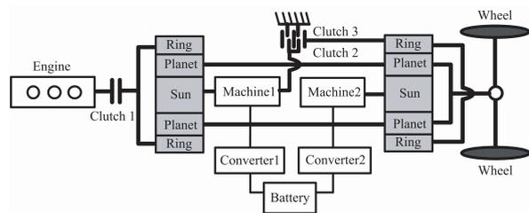
**Fig. 3** GM-Allison gear E-CVT propulsion system
