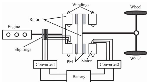
**Fig. 8** Axial-field double-rotor integrated PM machine gearless E-CVT propulsion system
