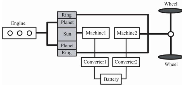
**Fig. 1** Toyota gear E-CVT propulsion system
