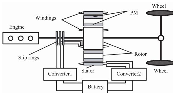
**Fig. 7** Double-rotor integrated PM machine gearless E-CVT propulsion system
