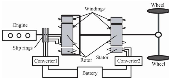
Fig. 4 Double-rotor cascaded induction machine gearless E-CVT propulsion system
