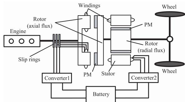
**Fig. 9** Decoupling double-rotor integrated PM machine gearless E-CVT propulsion system
