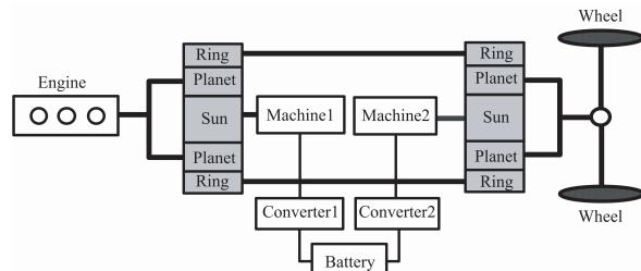
**Fig. 2** Ford gear E-CVT propulsion system
