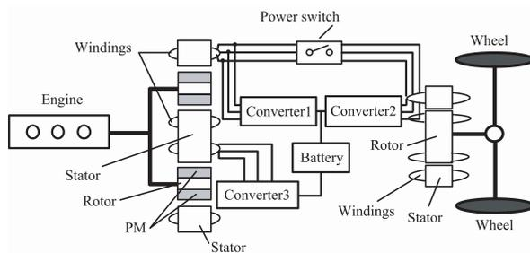
**Fig. 10** Double-stator PM brushless machine gearless E-CVT propulsion system
