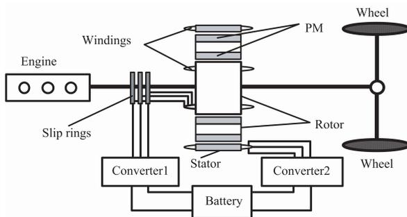
**Fig. 7** Double-rotor integrated PM machine gearless E-CVT propulsion system
