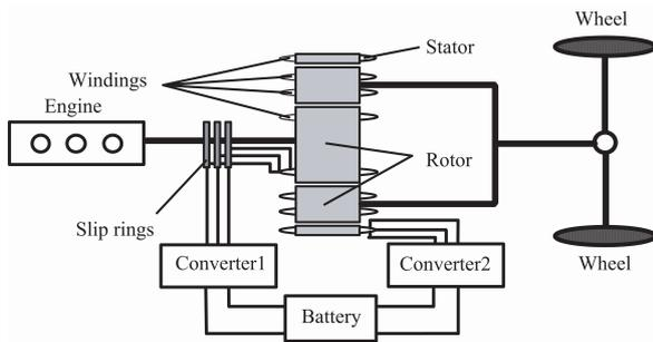
**Fig. 6** Double-rotor integrated induction machine gearless E-CVT propulsion system
