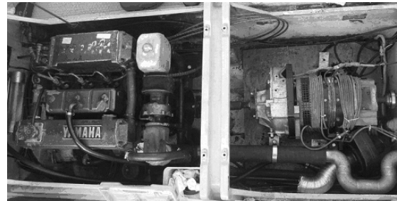
Fig. 8 Photographs of the PHEB drive-part after the propeller-shaft was replaced with an electric motor.
