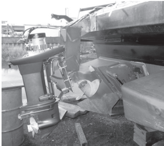
Fig. 1 A photograph of the tested boat and the temporarily installed electric outboard motor
