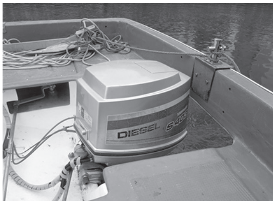
Fig. 6 A photograph of the unique diesel outboard motor
