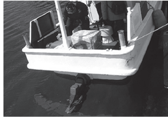
Figure 10: A photograph of the propeller propulsion system at the tail of the boat, PHEB-2
