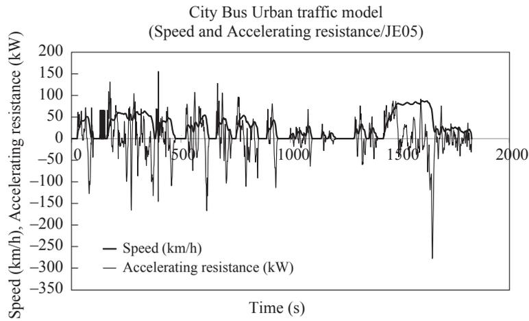
**Fig. 5** Acceleration resistance loss from one running
