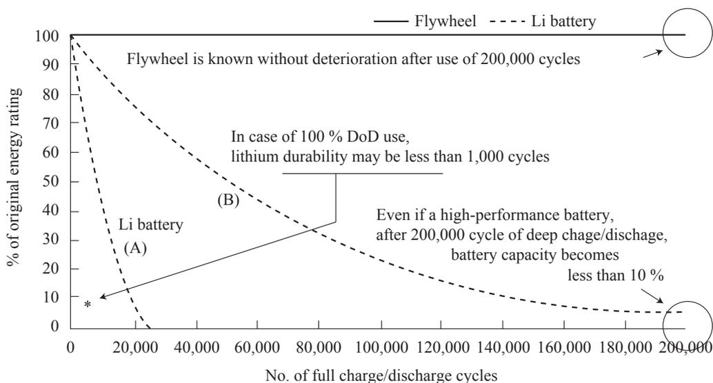
**Fig. 10** Performance of fly wheel versus li-ion battery for full charge/discharge cycles
