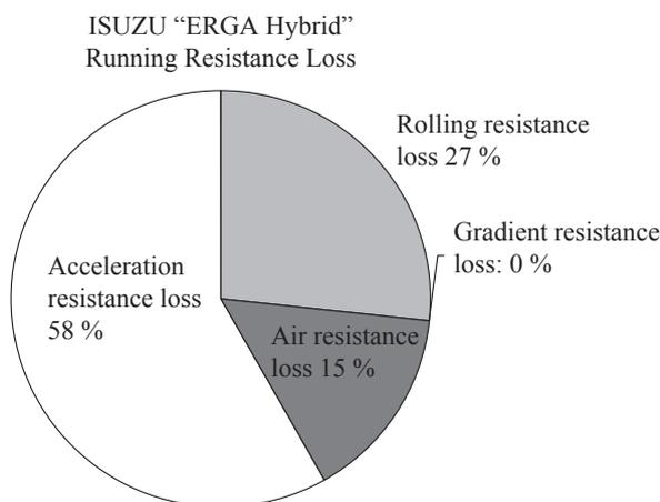
**Fig. 4** Itemized running resistance loss of an Isuzu ERGA Hybrid
