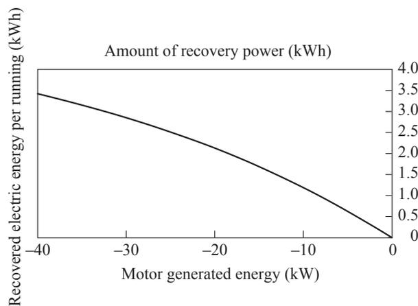
**Fig. 9** Amount of recovered electric energy per running in JE05 mode
