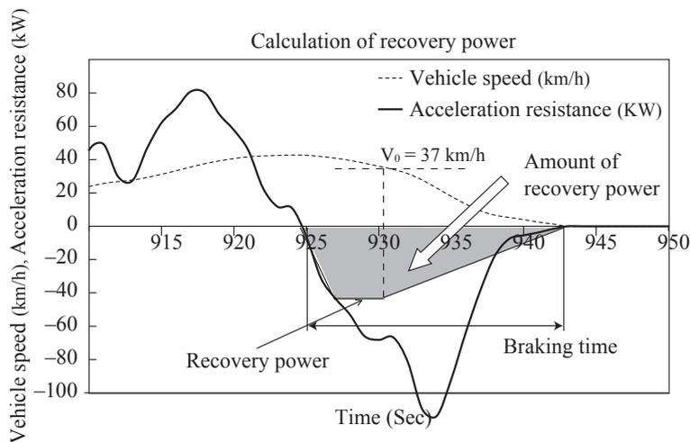
**Fig. 8** Regenerative cooperation braking
