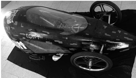
Fig. 20 Fabricated prototype three-wheel battery electric vehicle
