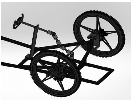
Fig. 8 Vehicle steering system
