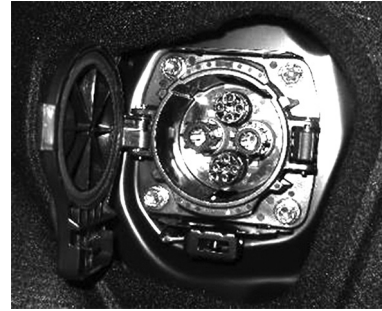
Fig. 8 An example of a CHAdEMO terminal loaded (Toyota “Mirai”) on a vehicle as a standard
