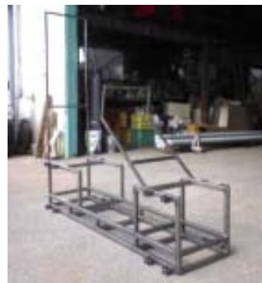
Fig. 11 Welded frame assembly
