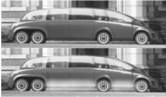
Fig. 19 The battery content is visualized by the form characteristic of an ‘EV Light Line’ at the side
