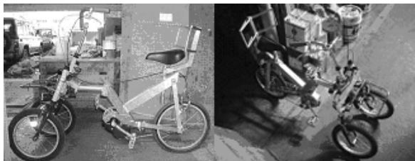
Fig. 9 Fabricated motor-assisted tricycle
