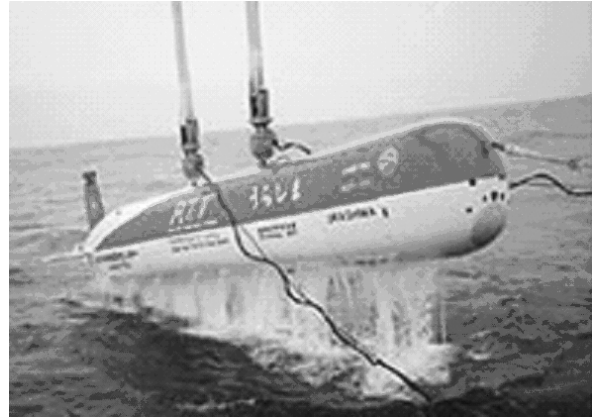
Fig. 5 A photograph of an unmanned vehicle which is a robot submarine for deep sea exploration [after Yamamoto et al., 2004]
