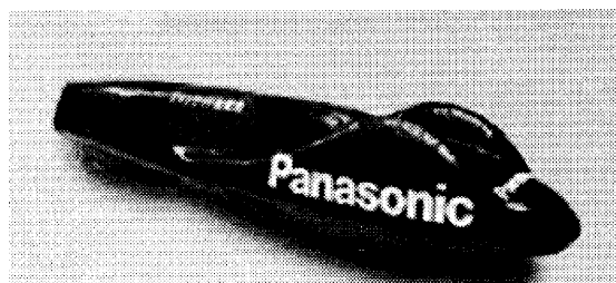
Fig. 1 A compact electric car run by 2 size-AA Oxyride dry-cell batteries (2004)
