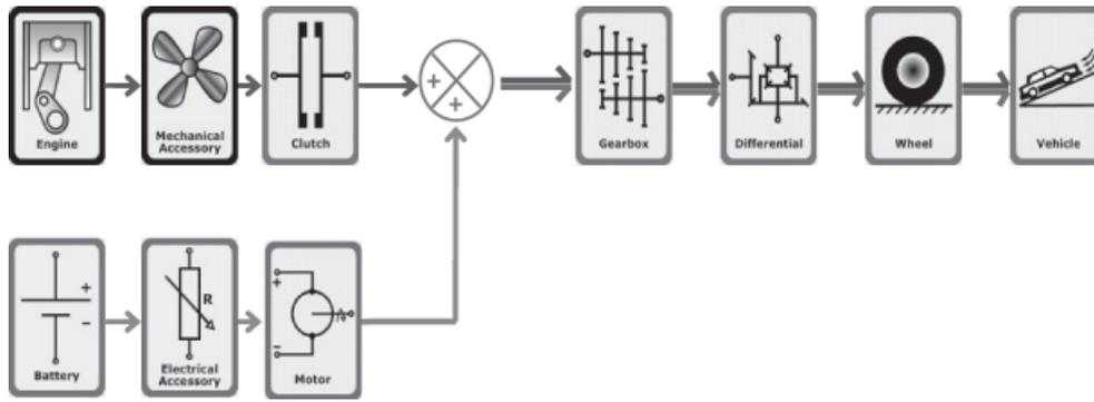
Fig. 2 Configuration selected – pre-transmission parallel HEV
