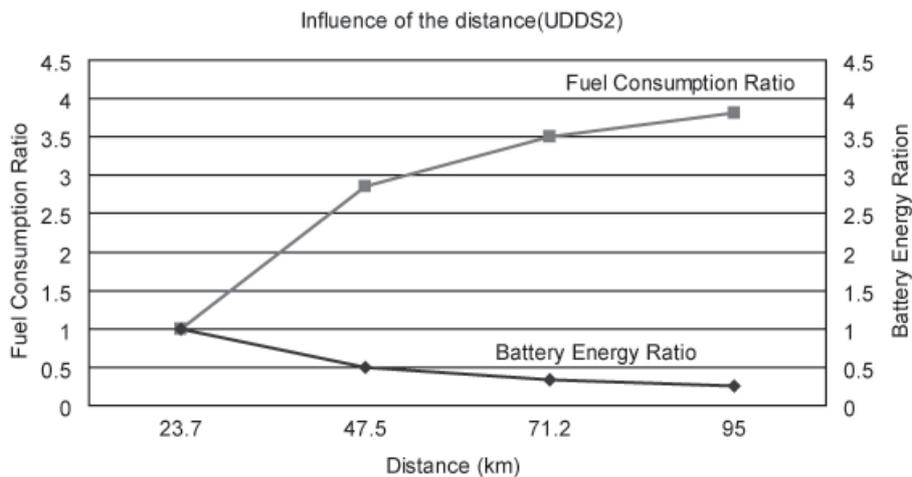
**Fig. 9** Fuel consumption and battery energy ratios on different distances based on optimized parameters from 2\*UDDS
