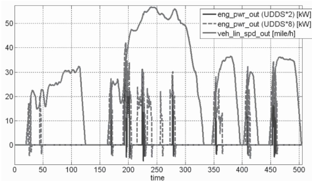
Fig. 6 Engine power for 2 and 8 UDDS
