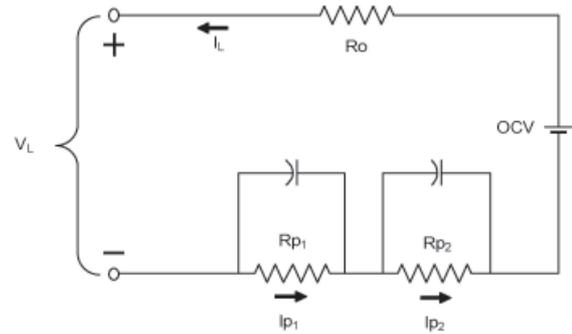
**Fig. 1** Battery electric circuit model
