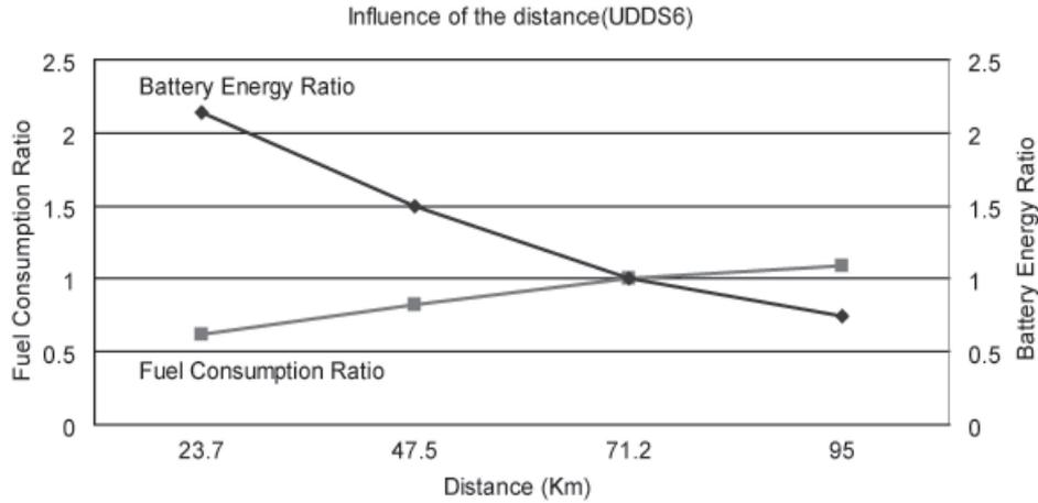
**Fig. 10** Fuel consumption and battery energy ratios on different distances based on optimized parameters from 6\*UDDS
