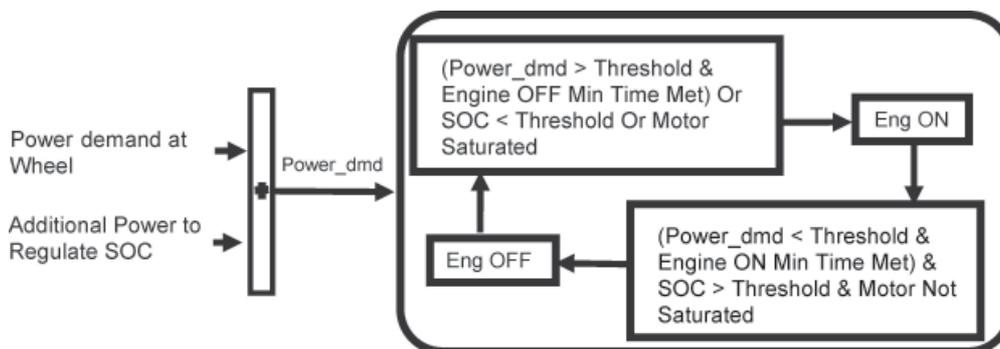
Fig. 4 Simplified engine on/off logic
