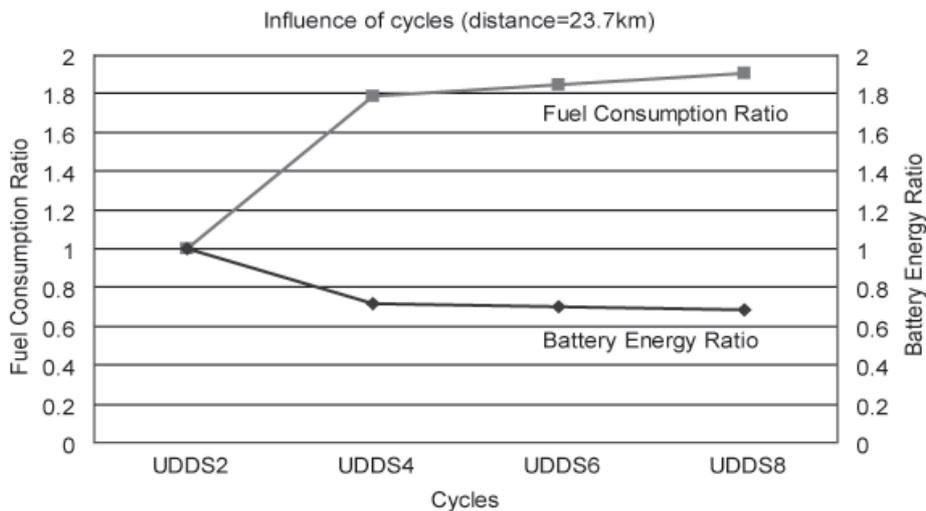
Fig. 7 Fuel consumption and battery energy ratios on 2\*UDDS
