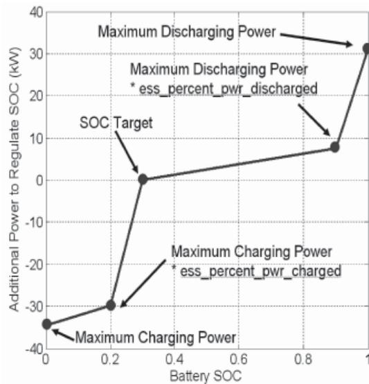
**Fig. 5** Example of additional power to regulate SOC
