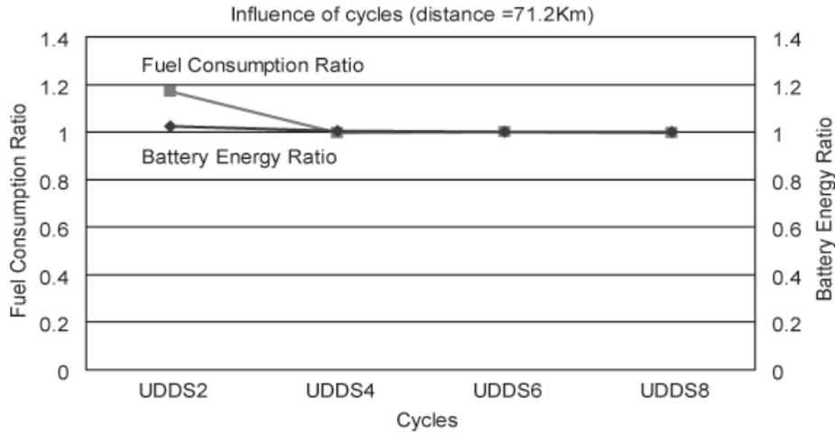
**Fig. 8** Fuel Consumption and battery energy ratios on 6\*UDDS
