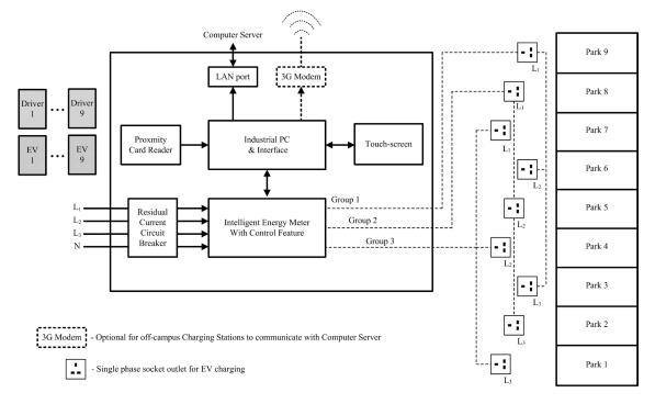
Fig. 6 Schematic of the EV charging station
