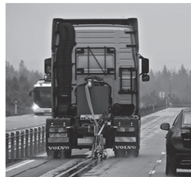
Fig. 2 Field test of the current collector, taken from Aldammad et al. (2014b)
