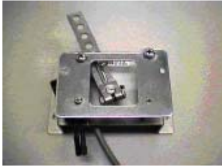
Fig. 13 The potentiometer for speed control
