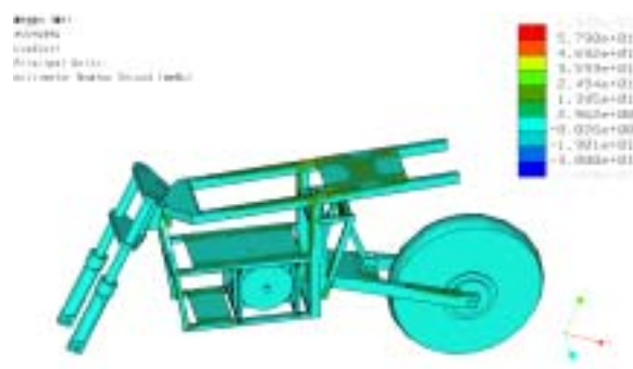
Fig. 10 A result of FEM stress analysis
