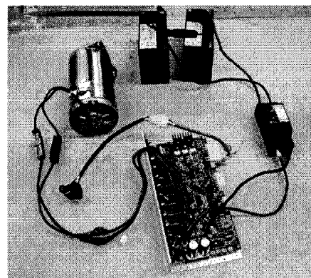
Fig. 10 Experimental equipment for control using potentiometer
