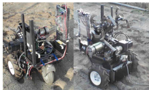
Fig. 5 Electric power tiller for house gardening, tiller work (left) and turning (right)
