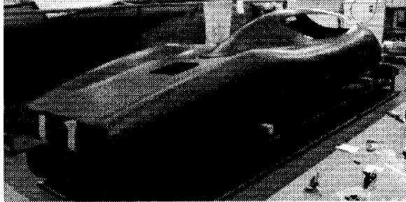
Fig. 10 CFRP-made lower part and upper part of the body
