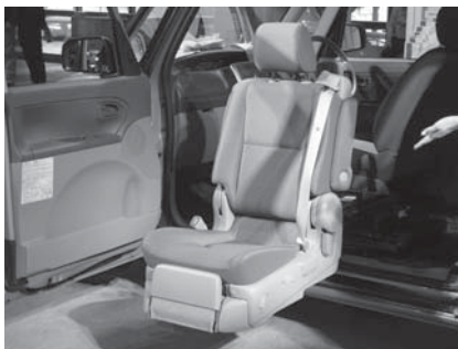
Figure 4-20 A lift-up passenger-seat (Daihatsu Motor)
