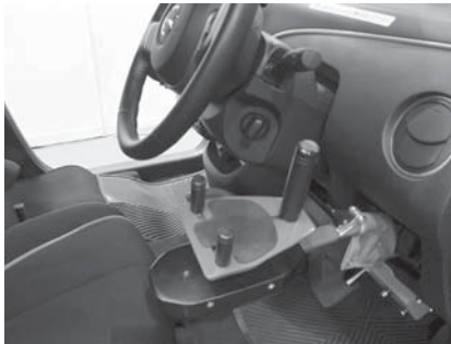
Figure 4-9 A joystick type assist-device for driving (Fuji Auto)
