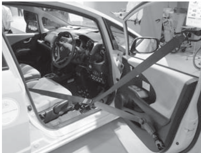
Figure 4-16 A device which helps the driver fasten the seat-belt automatically
