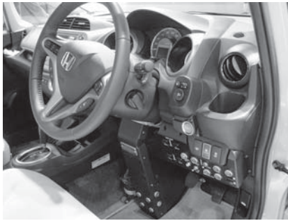
Figure 4-15 Combination switches for the foot
