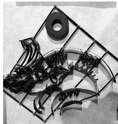
Figure 1: Traditional metal mold used for patterned washi
