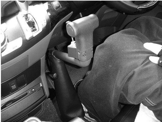
Figure 1: A general type of manual operation-device (Floor-type)
