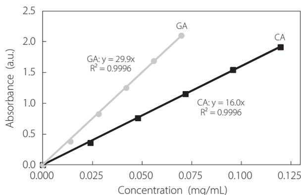
Figure 7: Calibration curve of CA and GA using micro-plate reader (ChroMate 4300)
