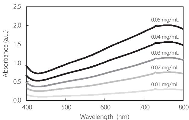
Figure 4: UV-Vis absorption spectrum of GA
