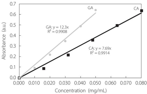
Figure 8: Calibration curve of CA and GA using digital camera (Nikon D70s)
