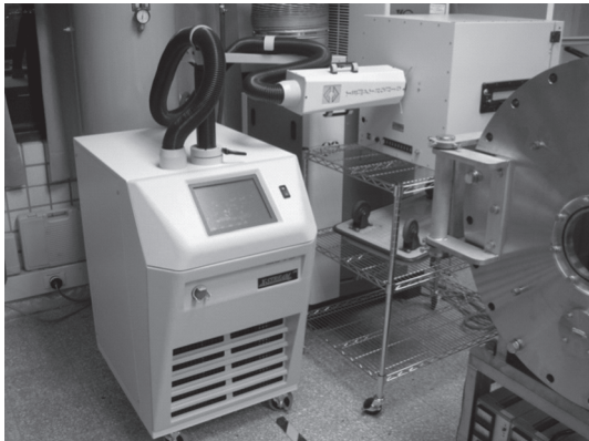
Figure 7: A thermal source for thermal vacuum test and temperature cycling test.
