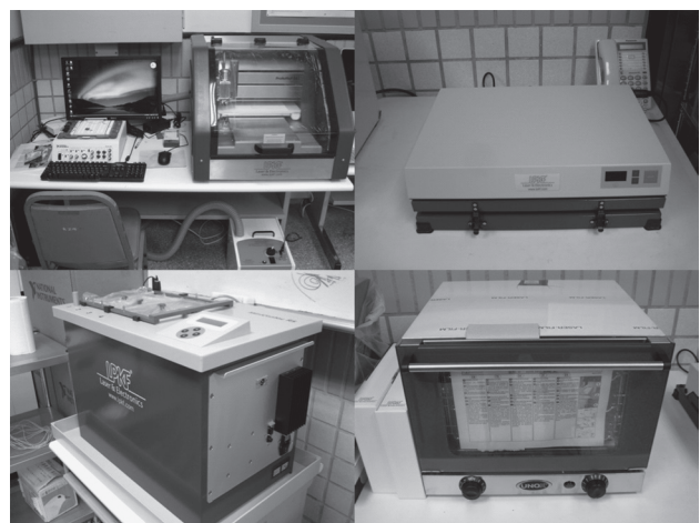
Figure 10: PCB circuit plotter (top left), UV exposer (top right), through-hole plating (bottom left), and hot air oven for solder resist mask (bottom right).
