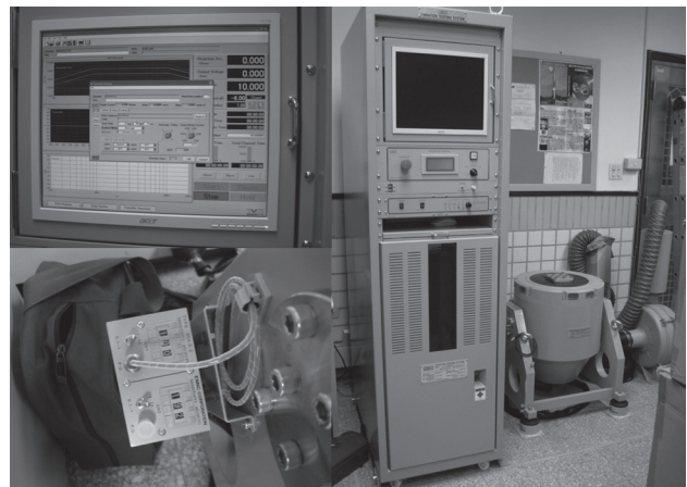
Figure 9: Vibration test system for sine and random vibration.
